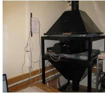
SEVAN Detector in mountain Mussala, research station of institute for Nuclear Research and Nuclear Energy; Bulgaria Latitude: 42° 10' 45.07" N Longitude: 23° 35' 6.96" E Altitude: 2926 m. a.s.l. Rc : 6.19 GV
