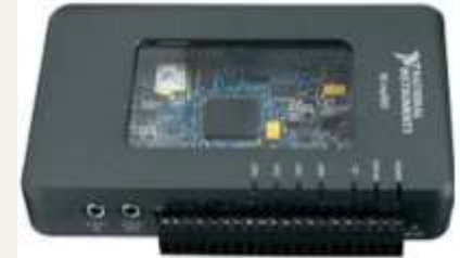
NI MyRIO board with GPS timing
