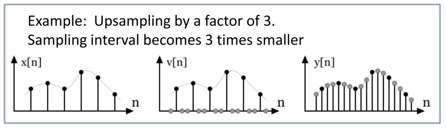
Upsampling produces an approximation of the sequence that would have been obtained by sampling the signal at a higher rate
