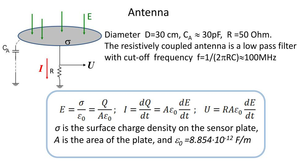
The resistively coupled antennas sense the time derivative of the incident electric field, dE/dt, and hence partially compensate for the falloff of lightning's VHF spectrum with increasing frequency
