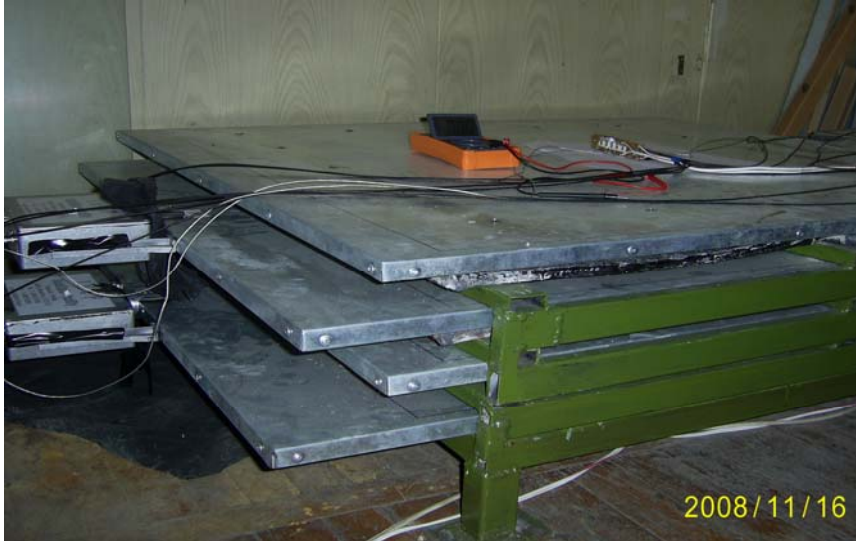
Figure 15 4-fold scintillator Detector assembly
