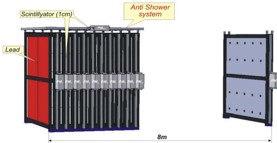
Figure 14. Setup of Horizontal Electromagnetic Calorimeter (HEC)
