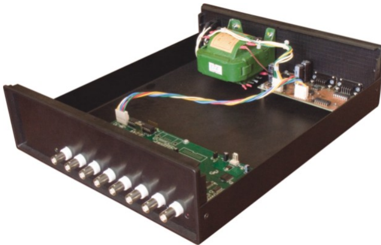
Figure 21 8 channel DAQ electronics for SEVAN detector
