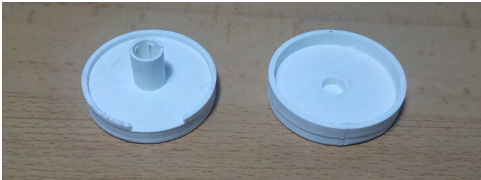
Figure 5.2.2: Printed casing tolerance tests
