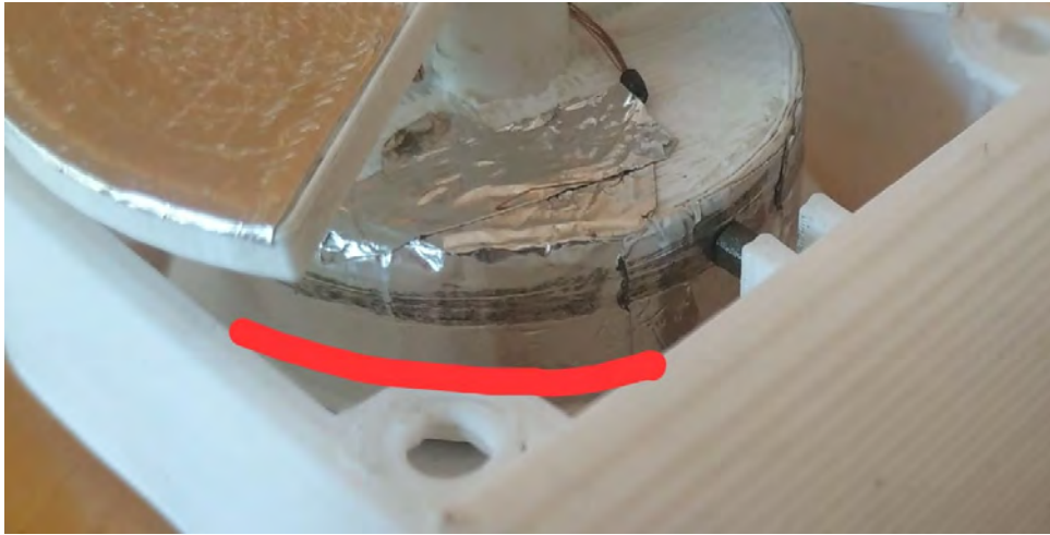
Figure 5.2.7: Detail of the contact area between the brush and the rotor casing
