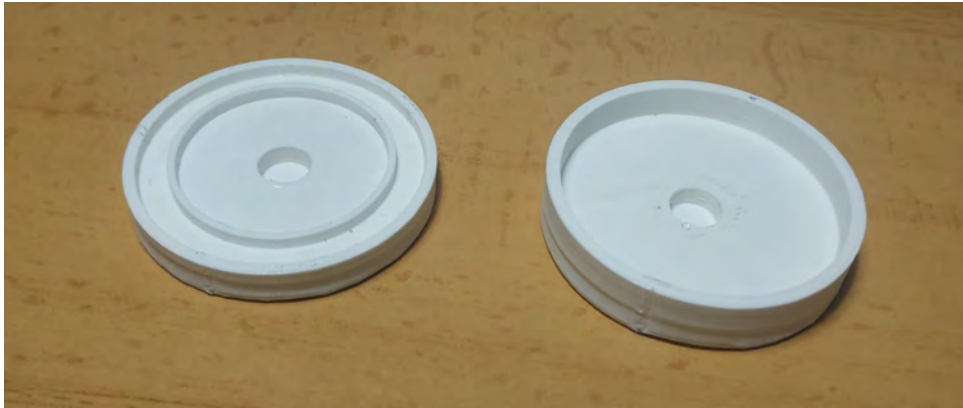
Figure 5.2.3: Change in the printed rotor casing
