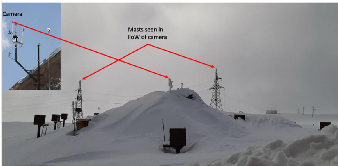
**Figure 9.** The MAKET experimental hall in winter, in the inset the zoomed ALL SKY CAM surrounded by DAVIS weather station, BOLTEK’s electric field sensor, and lightning tracker.
