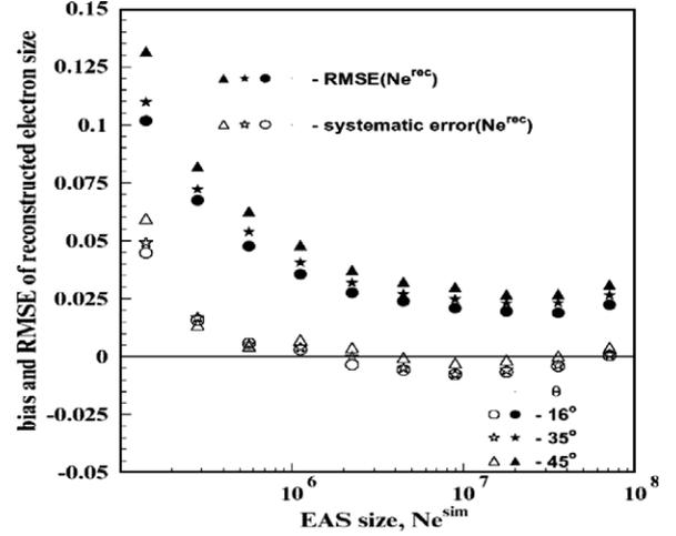
Fig. 9. The systematic errors and RMSE of shower size  $N_e^{\text{rec}}$  for different zenith angles of incidence.
