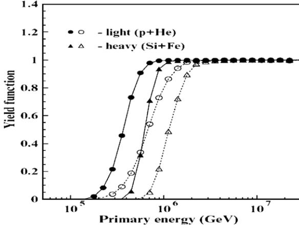
Fig. 8. The response of the MAKET-ANI detector on simulated “light” (p + He) and “heavy” (Si + Fe) induced showers, versus primary energy; shower selection criteria:  $N_e \geq 10^5$ ,  $\theta \leq 30^\circ$  (closed symbols),  $N_e \geq 10^5$ ,  $30^\circ \leq \theta \leq 45^\circ$  (open symbols).
