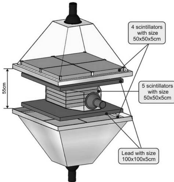
**Fig. 2** Basic detecting unit of the SEVAN network
