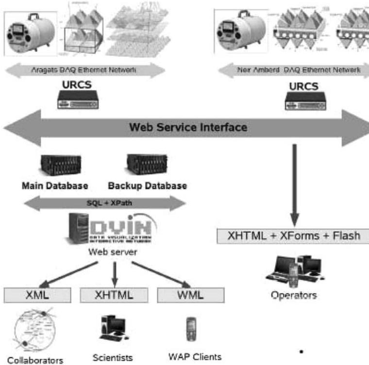
**Fig. 4** Layout of the new ASEC data acquisition system. Several detector arrays are operating at Nor-Amberd and Aragats research stations. The detectors are controlled by URCS which are installed on each station. The data dissemination and detector control is performed by web services. The DVIN is used to distribute the data to end users
