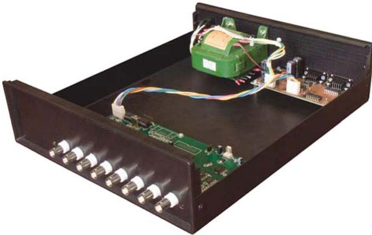
**Fig. 3** Eight channel DAQ electronics for SEVAN detector
