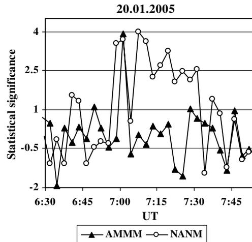
Fig. 5. Comparison of the time series of the 3 min count rates measured by ANM and AMMM detectors expressed in the units of the standard deviations. Duration of the peak measured by AMMM is  $\sim 3$  min, whereas excess of ANM count rate is much longer  $\sim 45$  min.
