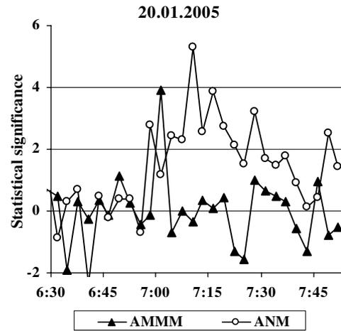
Fig. 4. Comparison of the time series of the 3 min count rates measured by NANM and AMMM detectors expressed in the units of the standard deviations. Duration of the peak measured by AMMM is  $\sim 3$  min, whereas excess of ANM count rate is much longer  $\sim 45$  min.
