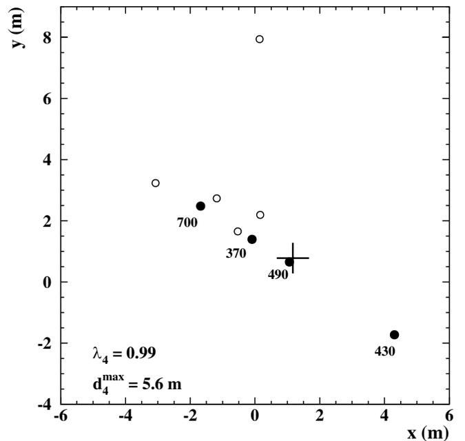
FIG. 1. Example of a measured hadronic shower core (hadron positions in the shower plane) with  $\lambda_4 = 0.99$  and  $d_4^{\max} = 5.6$  m. 9 hadrons with energies above 100 GeV are reconstructed. For the four most energetic hadrons (full symbols), the energies in GeV are given. The shower core position as reconstructed by the scintillator array is marked by a cross. The active calorimeter area exceeds the area plotted.
