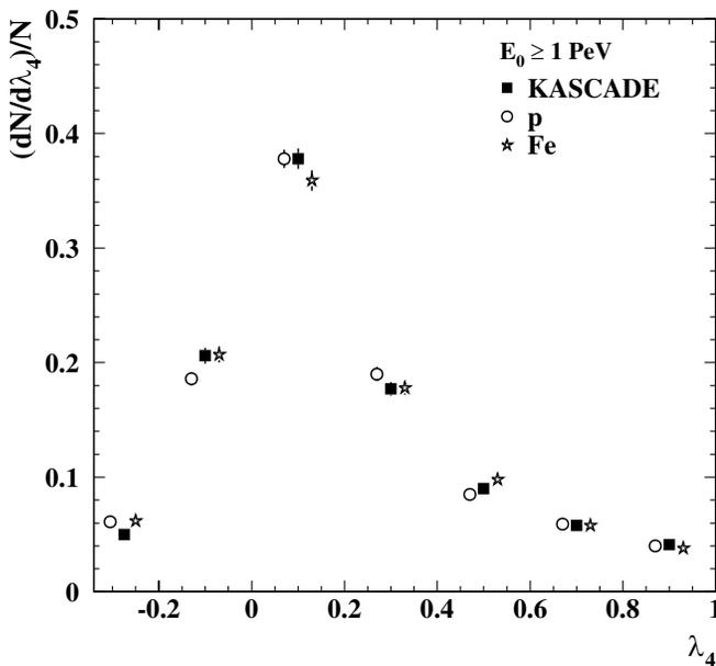
FIG. 2.  $\lambda_4$  distribution measured by KASCADE compared to simulation results for primary proton and iron showers. For clarity, simulation points are slightly displaced horizontally.
