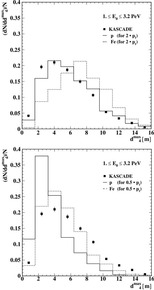
FIG. 8.  $d_4^{\max}$  distribution measured by KASCADE (see Fig. 7) compared to simulation results for primary proton and iron showers with modified transverse momentum of secondary hadrons. The transverse momenta were artificially increased (upper panel, “ $2 \cdot p_t$ ”) and reduced (lower panel, “ $0.5 \cdot p_t$ ”) by a factor two.
