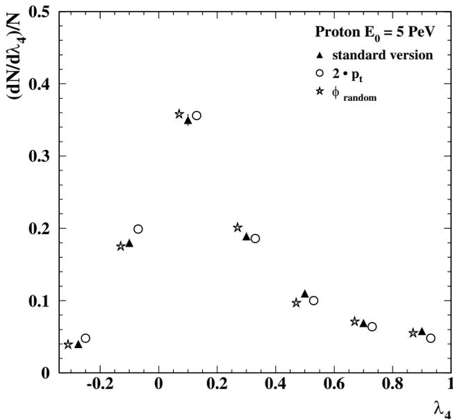
FIG. 4.  $\lambda_4$  distributions for proton showers of 5 PeV primary energy without modification of the hadronic particle production (“standard version”), with randomly chosen azimuth angles of secondary hadrons (“ $\Phi_{\text{random}}$ ”), and with transverse momenta of secondary hadrons increased by a factor two (“ $2 \cdot p_t$ ”). Simulation points obtained after the modifications are slightly displaced horizontally.
