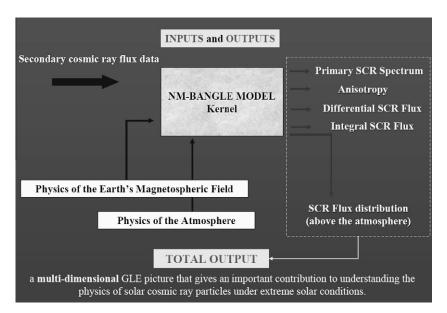
Fig. 4. Inputs and outputs of the NM-BANGLE model.
