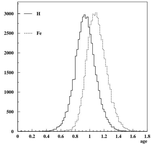
Figure 5: The shower age parameter of proton and iron for the MC data including detector response
