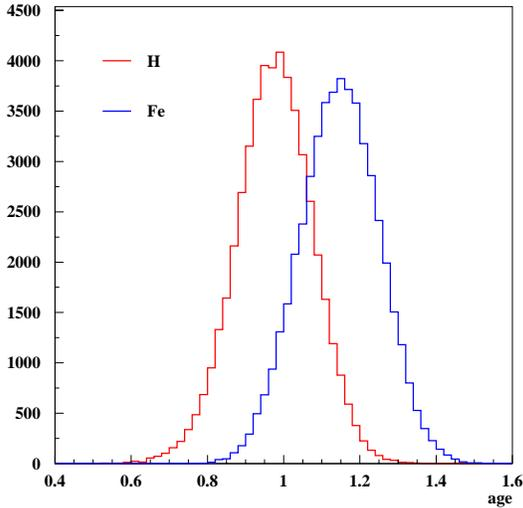
Figure 4: The shower age parameter of proton and iron for the MC data without detector response
