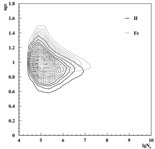
Figure 7: *The shower age versus shower size  $f$  proton and iron for the MC data with detector response*
