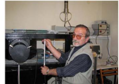
Figure 6 Gagik Hovsepyan checking the gap in the SEVAN detector
