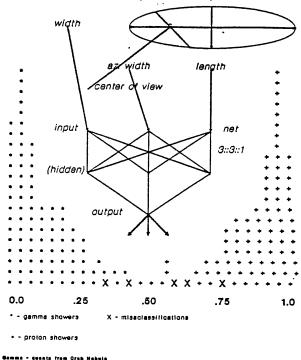
The input of each neuron (excepts the first input layer) consists of the weighted sum of outputs of previous layer neurons:
