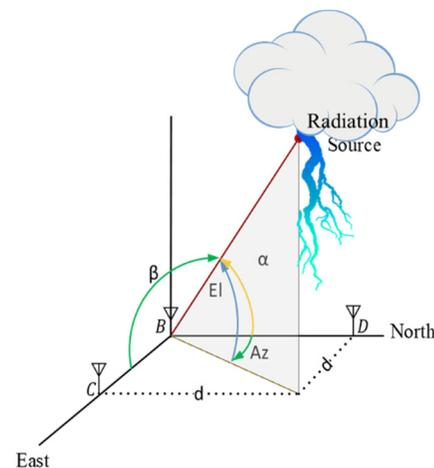
FIGURE 4. Two-orthogonal baseline schematic diagram of 2D ITF lightning location system.
