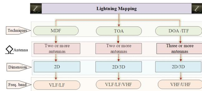
FIGURE 1. Lightning mapping methods.
