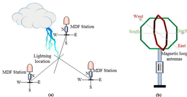
FIGURE 2. Lightning detection using MDF. (a) Multistation MDF; (b) orthogonal magnetic antenna.
