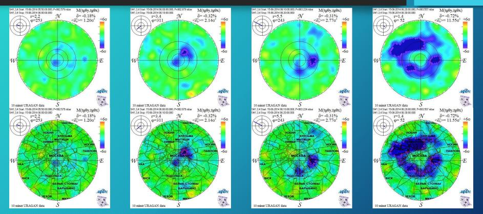
Muonograph is a graphical representation of the variations matrix of counting rate angular distribution over the last 10 minutes with respect to the normalization matrix of the preceding 24 hours in statistical error units
