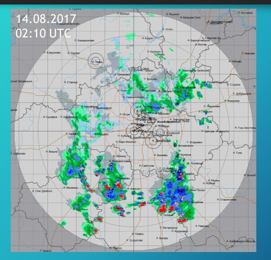
DMRL provides cyclic monitoring at 10 minutes intervals and obtains data with a high spatial resolution (1 km  $\times$  1 km). Radar operates by conducting a survey sequence of circular azimuthal scans of the upper celestial hemisphere at several different angles. By doing so it collects data on cloudiness and precipitation on several conical sections of the atmosphere.
