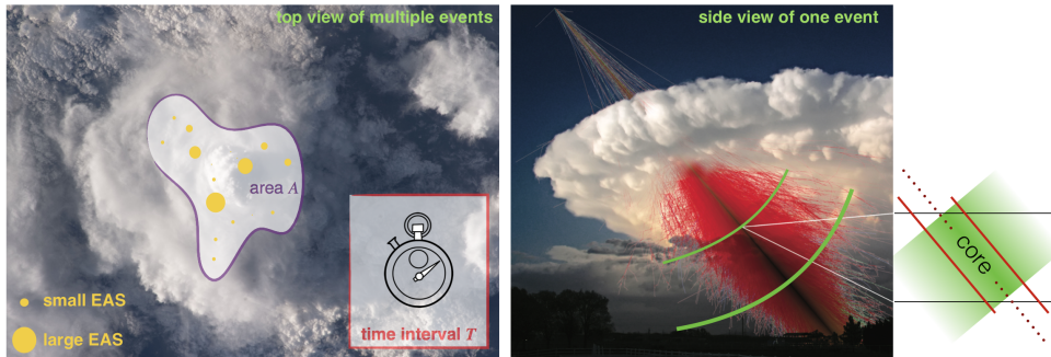
Figure 11.2: Illustration of the system. Left panel is the top view of a thundercloud, where within a certain area A and time interval T of interest multiple EAS events take place. Some small, some large, randomly distributed in time, location and size, but we assume that they do not interact or overlap. Right panel is the illustration of the side view of one single event. In red the time integrated paths of the particles of the extensive air shower. In green are two snapshots in time to illustrate that it is actually a pancake structure moving with almost the speed of light towards the ground. Around the axis (the momentum vector of the initial cosmic ray) particles are concentrated in a dense core.
