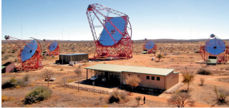
Figure 3.5: The H.E.S.S. instrument located in Khomas Highland in Namibia. The system is composed of four smaller and one large IACT. The control building (front) and the telescope camera shelters in front of each telescope can be seen. (Image credit: H.E.S.S. Collaboration)
