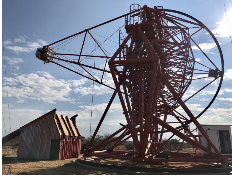
Figure 3.6: Side view of one of the H.E.S.S. telescopes (CT4). Cherenkov light illuminating the mirror dish, segmented in 382 circular mirror facets of 60 cm diameter, is focused on the 15 m distant Cherenkov camera (which in this image is protected from the daylight by its closed lid). The cabin, which holds the telescopes steering, monitoring and networking devices, is mounted to the back of the telescope. On the left hand side, the shelter, in which the Cherenkov camera is parked during day- and bad-weather time, can be seen. The telescope structure tracks on a circular rail to ensure homogeneous movement in the azimuth. Altitude tracking is steered via the semicircular structure on the back of the telescope dish. (Image taken in March 2019)
