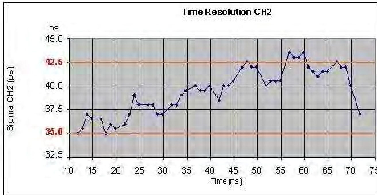
Fig.2 – Time resolution of the ToF electronics realized for the PAMELA experiment.
