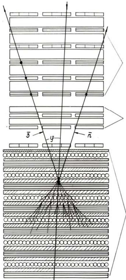
Ionization Calorimetry, particle energy up to 50 TeV; hadron identification with TRD; Computer DAQ – first Armenian mini computer – NAIRI.
