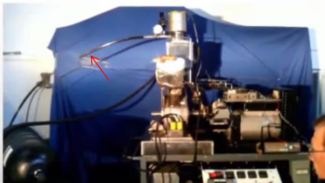
Figure 15 Stills from video of CES steam generator. A) shows the appearance before steam has emerged. B) shows the situation as the steam emerges. The steam in fully vapour and as such is invisible, but its presence is clear from the refraction of light from objects behind the steam. c) The steam cools and the water vapour condenses out into visible droplets.
