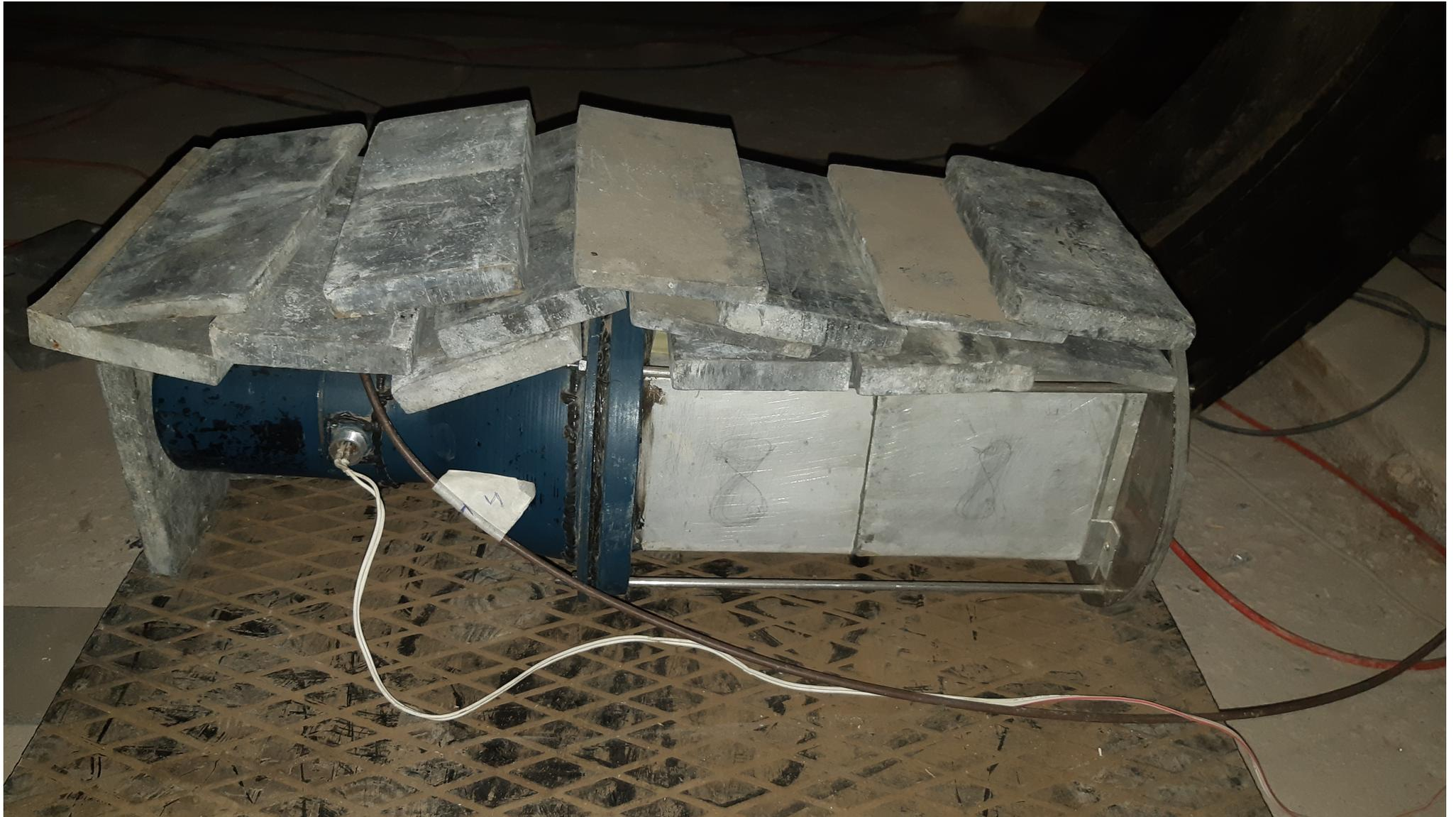
**Nal N1 open from all sides, top and bottom. Can register RREA, MOS and flux from the bottom (if any)**
