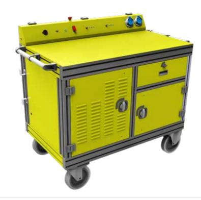
The Baykar Ground Support Unit (GSU) powers the Bayraktar TB2 Platform on the ground, charges smart batteries, and provides maintenance via an operator interface. The GSU can charge batteries or the UAV for four hours without needing an external power source. When plugged in, it operates on a standard 220-230V AC source and has wheels for easy mobility.
