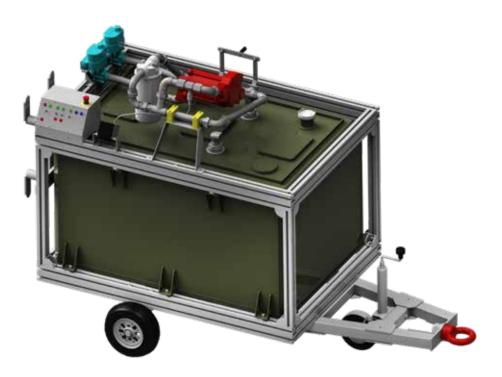
The Baykar refueling station is custom-made for the Bayraktar TB2 platform and comes with an 800 litre capacity in semi-trailer form factor. The station can both refuel and defuel the aircraft.
