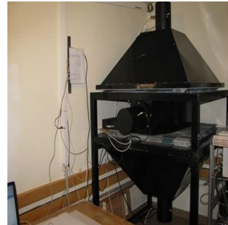
Figure 3. SEVAN Detector in Mussala mountain research station of Nuclear Physics Institute of Bulgarian Academy of Sciences
