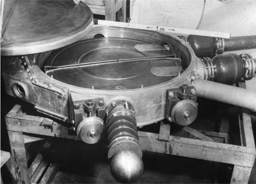
ILLUSTRATION 49 Kaiser Wilhelm Institute for Medical Research, Bothe's Institute for Physics, Heidelberg. The cyclotron vacuum chamber where particle trajectories are bent by the magnetic field and repeatedly accelerated by an electric field.
