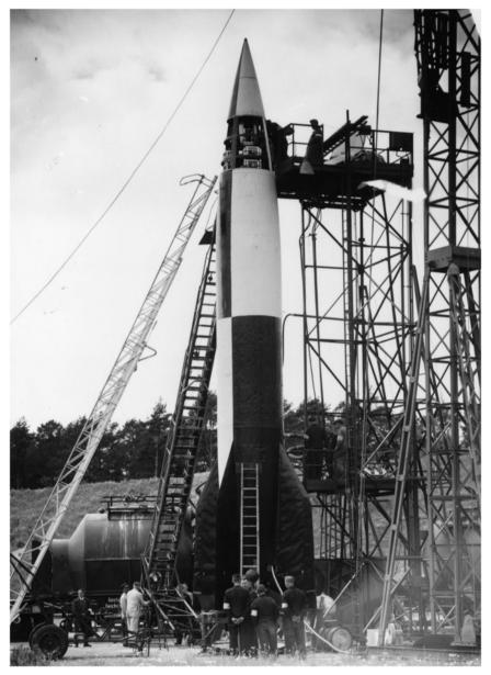
ILLUSTRATION 70 Preparation for the launch of an A-4 rocket, 1942: the control section of the world's first large rocket to travel in space, which was 14 meters high and weighed 12.9 tons with full tanks, is open; above there is space for a payload of one ton. The A4 missile (A stands for Aggregate), a series of ballistic rockets developed by Wernher von Braun's group in Peenemünde, was later named the V2, Vergeltungswaffe (weapon of retaliation).
