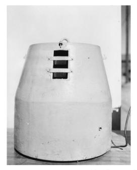
ILLUSTRATION 69 Rare image of the fully equipped 'Regener Tonne,' the first scientific rocket payload designed to reach the upper part of the atmosphere. This image was found by chance by the engineer Gerhard H. R. Reisig, who had been in charge of the instrumentation and measurement parts of the instrument. The project, developed in the early 1940s, was under
