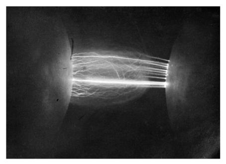
ILLUSTRATION 43 Van de Graaff accelerator: flashover due to electric discharge of high current made through the air between the spheres at very high electric potential.
