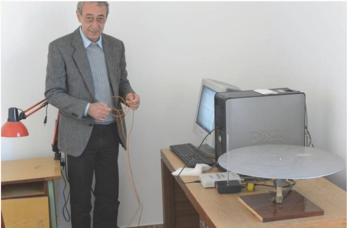
Figure 1. Suren Sogomonyan near new installed on Aragats fast electric field monitoring system. Measurement system involves flat plate antenna followed by a passive integrator, and a digital storage oscilloscope with 10 ns sampling interval.
