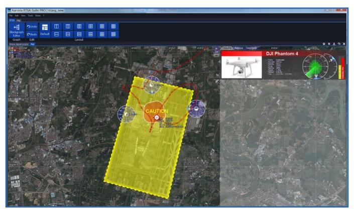
This picture shows the map view of the AARTOS DDS, with triangualted position of the drone (red) inside a warning area (yellow). The DDS shows even the type of detected drone and can handle an unlimited number of drones simultaneously.
