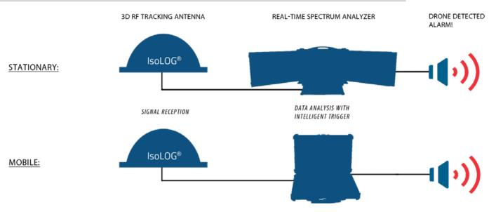
The single site solution is ready to use within a few minutes only. Based on a stationary or mobile Spectrum Analyzer (RF Command Center or XFR V5 PRO, see page 6) and the 3D direction finding antenna IsoLOG 3D, this solution is the first choice for surveillance of smaller areas, e.g. a house or a prison.
