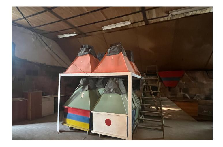
CUBE and STAND3 detectors operate on nanosecond to minute time scales to research the space temporal structure of TGE and measure electron and gamma ray energy spectra.
