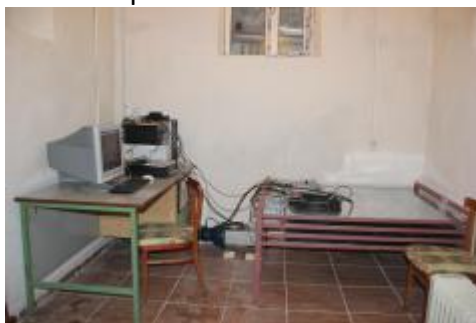
Figure 6 HEAR monitors: STAND1 and NaI particle detectors are measuring 1-minute time series (in the right); electronics and control equipment send data on-line each minute to Yerevan CRD headquarters (on the table).
