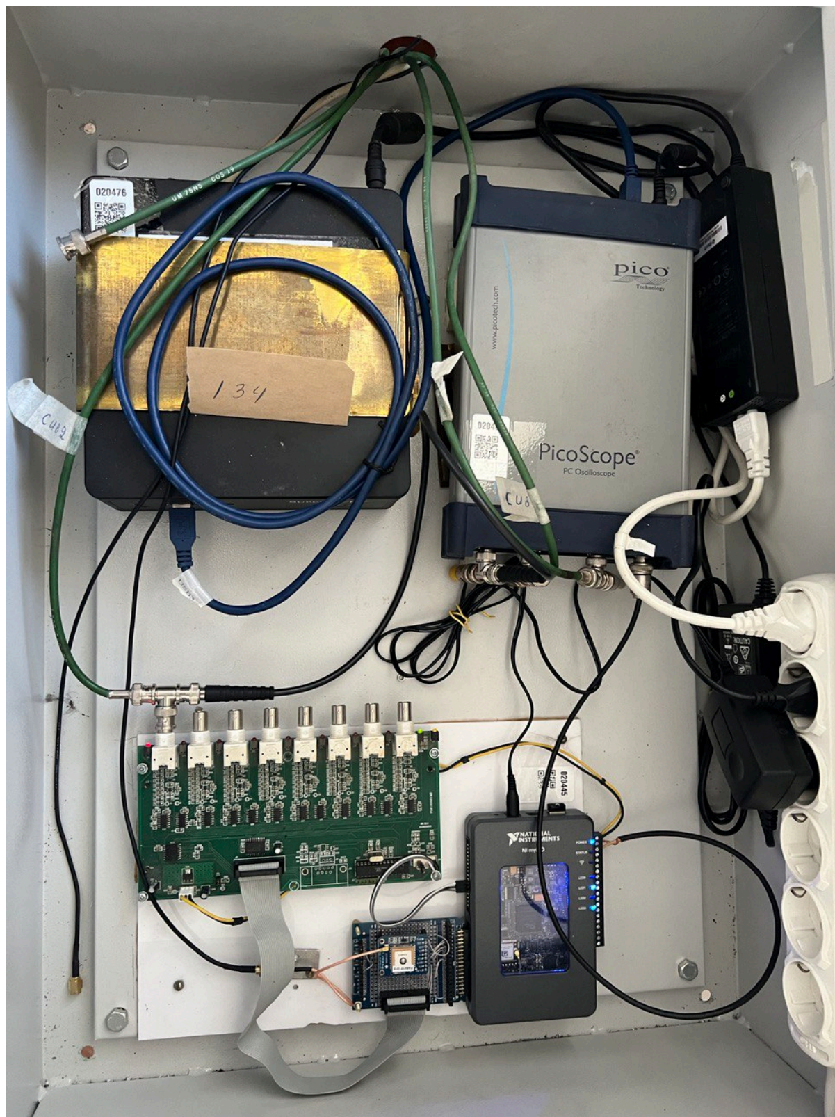
Figure 6. High-frequency oscilloscopes and National Instrument's boards allow synchronizing particle fluxes and atmospheric discharges on nanosecond time scales
