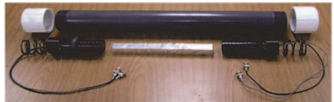
Figure 3. PVC assembly containing a BGO scintillator and 2 PMTs to view either end. Six of these are placed in each TETRA-II box.
