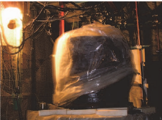
Figure 5. An old Germanium detector (surrounded by shielding to decrease environmental background).
