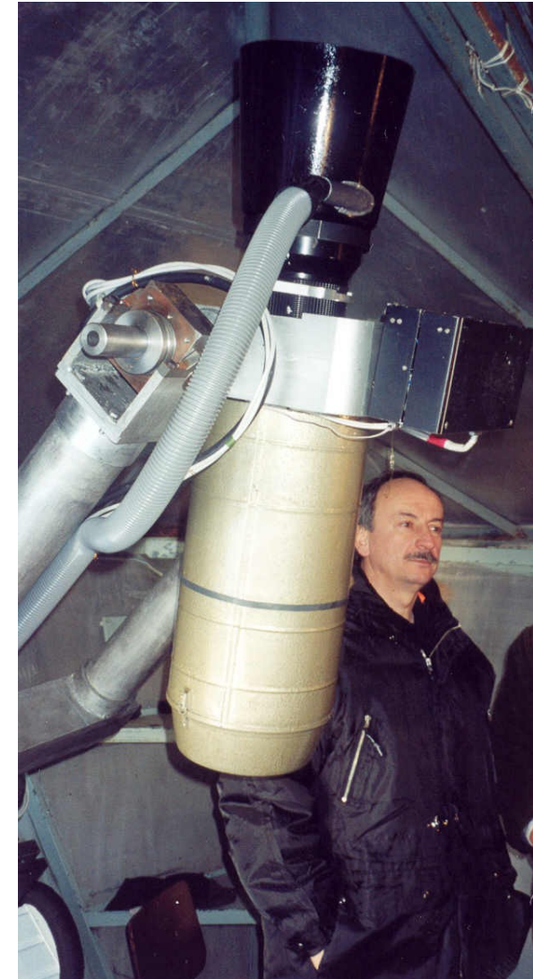
FAVOR (FAST Variability Optical REGISTRator) camera — SAO RAS, since 2003 Built in collaboration with IPI and IKI (Moscow), supported by CRDF grant
