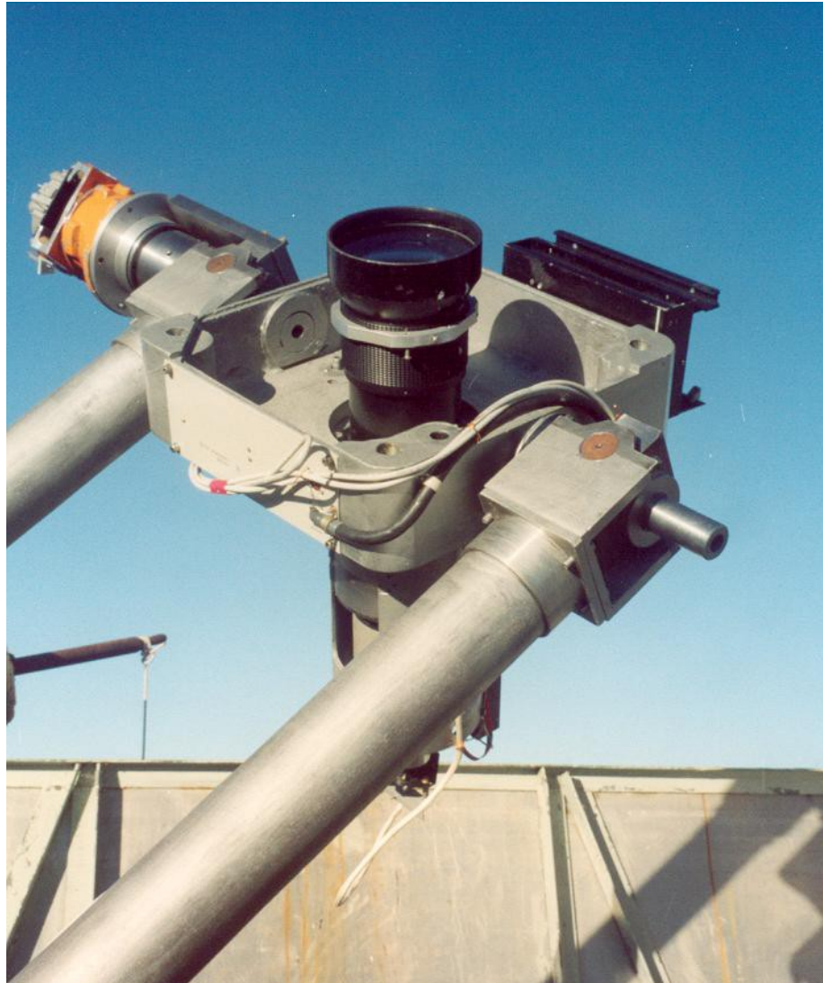
FAVOR (FAST Variability Optical REGISTRator) camera — SAO RAS, since 2003 Built in collaboration with IPI and IKI (Moscow), supported by CRDF grant
